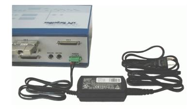
8 Plug the socket end of the cable into the external AC power adapter.
