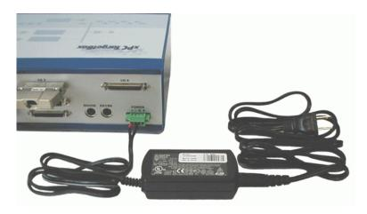
You are now ready to start the xPC TargetBox for self-testing. Because the xPC TargetBox does not have a power switch, the system starts to operate as soon as you plug the AC power cord into a wall outlet.
