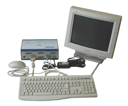
The next step is to connect the xPC TargetBox to a host computer using either a serial or network connection. See "Host PC to xPC TargetBox Communication" on page 3-12.
